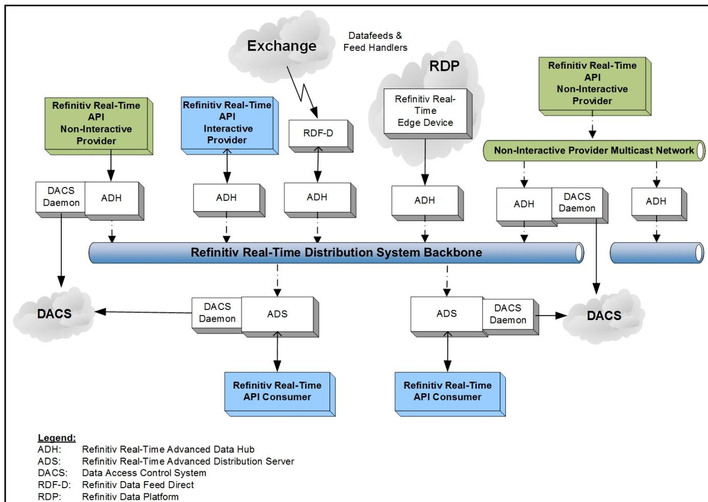
Figure 19. Typical Refinitiv Real-Time Distribution System Components
